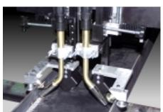
Mechanical torch tracking devices maintain proper torch position.
