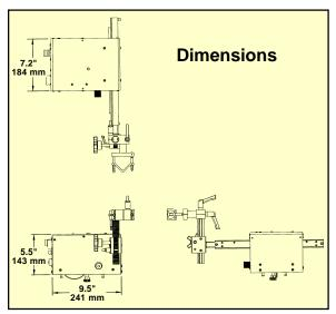
Input Voltage: BUG-5700 120 VAC 50/60Hz Travel Speed: 3-65 ipm (70 – 1670 mm/min.) Oscillation Speed: 4-98 ipm (100 – 2500 mm/min.)
