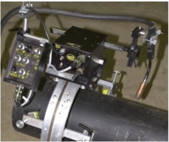
The **UNIVERSAL BUG-O-MATIC** is a compact unit which combines a powerful drive and precision oscillator all in one housing. The unit is lightweight and can easily be handled by one operator. The machine works in all positions and can be used for vertical and overhead welds. By simply changing the carriage, the unit can work on rigid rail, semi-flex rail, hi-flex rail or complete ring rails. The opening mechanism of the carriage allows the unit to be released or installed anywhere on the rail.
